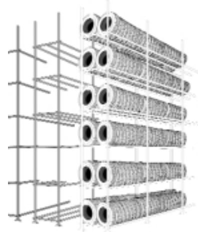
[On-Tread Storage Of Rubber Tires In Double Row Rack]
